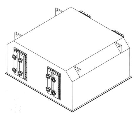
Figure 2 - Shroud / Air Guide Cover
